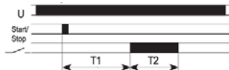
FZ41: Pulse generator with Start/Stop pushbutton
