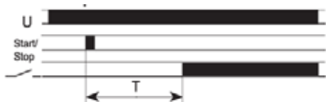
FZ38: On delay with Start/Stop pushbutton
