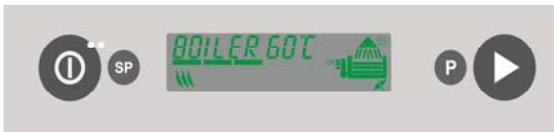
If your machine is equipped with an LCD, it will be necessary to make sure that the control board firmware is compatible with the pushbutton panel firmware.
