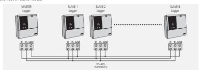
The master can display the data of any of the units connected to it and print them if the unit has a printer (it is recommended to use an AKO-15742 or 15752 as master).
