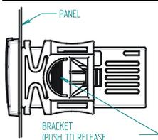
Instrument XR70CX shall be mounted on vertical panel, in a 29x71 mm hole, and fixed using the special bracket supplied. The temperature range allowed for correct operation is 0 to 60°C. Avoid places subject to strong vibrations, corrosive gases, excessive dirt or humidity. The same recommendations apply to probes. Let air circulate by the cooling holes.
