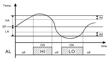
The maximum and minimum temperature alarms can be disabled by setting the relative parameters "HA" and "LA" = oF.
