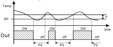
Third control (par. "P3") foresees an inhibition to the activation of Through par. "dL", "Et" and "dA" it's possible to define the display the output "Out" by a time delay that starts when the output was turning on last time (delay between switching-on).
