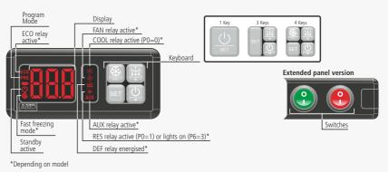
Flashing lights indicate that the function in question should be activated by temperature, but is not due to a conflicting timing or protection parameter.
