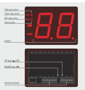
**Flashing** lights indicate that the function in question should be activated by temperature, but is not due to a conflicting timing or protection parameter.
