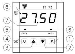
1 - Key P: Used for the set point setting and to program the functioning parameters
