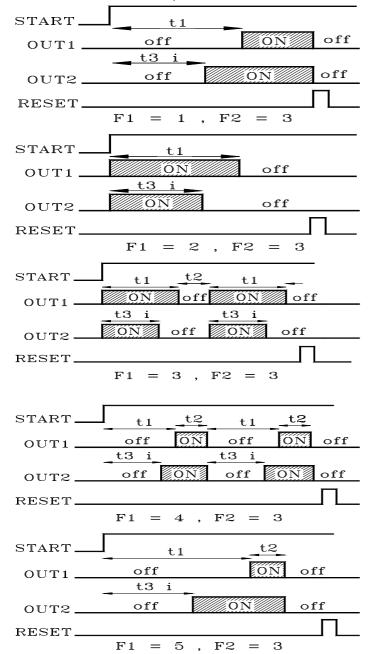
The output OUT2 exactly operates like the output OUT1 so that to F2 = 4 - Same function of OUT1 (time t1) with time t3 relative to t1 (in advance): The choice of this mode of operation enable the set "t3" that it has the same range time "S1" and cannot be higher of "t1."
