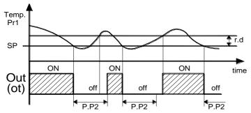
Third control (par. "P.P3") foresees an inhibition to the activation of the output by a time delay that starts when the output was turning on last time (delay between switching-on).
