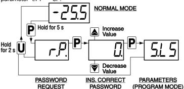
Note: If the Password gets lost, just swith off and on the instrument supply, push P key during the initial test and keeping the key pressed for 5 seconds.
