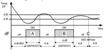
**Examples:** defrosting A ends due to reaching of temperature "dtE", defrosting B ends at the end of the "d.dE" time as the temperature "d.tE" is not reached, defrosting C does not take place as the temperature is higher than "d.tS".
