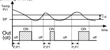
Second control (par. "P.P2" ) foresees an inhibition to the activation of the output by a time delay that starts when the output is turning off (delay after switching-off).
