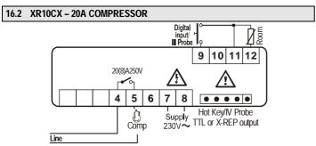
9-40Vdc supply: connect to the terminals 7 and 8.
