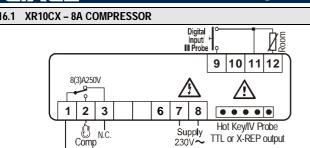
**9-40Vdc supply**: connect to the terminals 7 and 8. **12Vac/dc supply**: connect to the terminals 7 and 8. **24Vac/dc supply**: connect to the terminals 7 and 8. **120Vac supply**: connect to the terminals 7 and 8.
