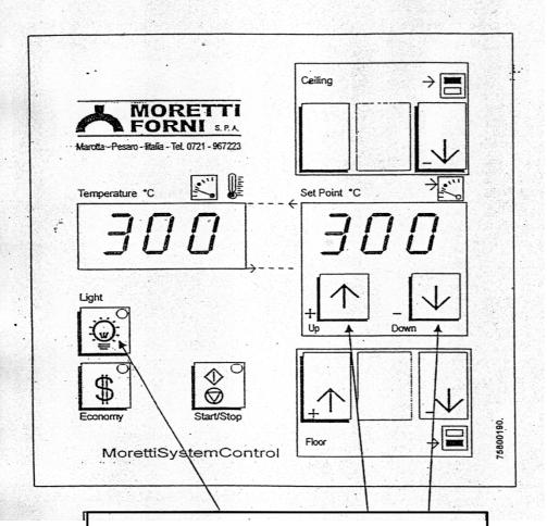
Push for 5 seconds to changing the setting of the contact of the safety thermostat.
