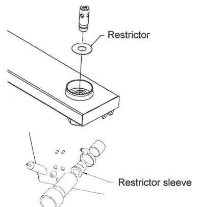
On machines built before 1991 the plastic restrictor sleeve should be mounted at the connection end of the flushing system.
