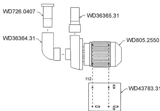
Adapter WD43783.31 is not to be used if the machine is fitted with pump FIR 0251.
