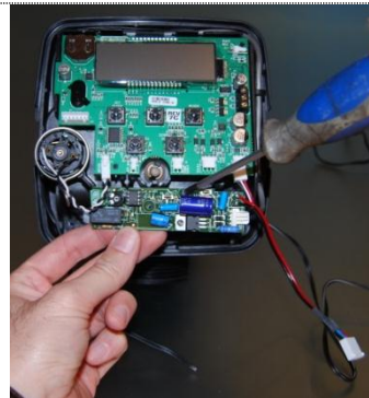
THREAD THE CABLE TO CELL TITANIUM
