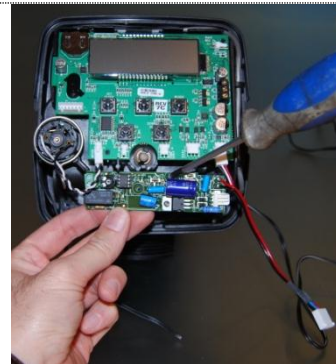
THREAD THE CABLE TO CELL TITANIUM
