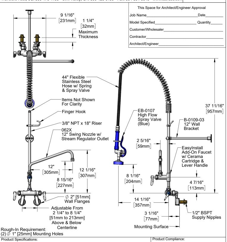
International Pre-Rinse Unit: Wall Mount Mixing Faucet, Quarter-Turn Cerama Cartridges w/ Check Valves, Lever Handles, 44" Flexible Stainless Steel Hose, High Flow Spray Valve (Blue), Add-On Faucet w/ Cerama Cartridge & Lever Handle, 12" Swing Nozzle, 12" Wall Bracket & 1/2" NPT Female Adjustable Flanges w/ 1/2" BSPT Male Supply Kit
