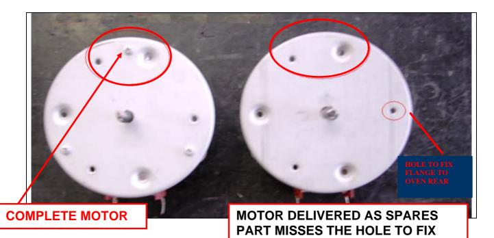
IF POSSIBLE, DISMANTLE THE ORIGINAL FLANGE AND MOUNT IT ON THE NEW MOTOR, OTHERWISE DRILL OUT THE MISSING HOLE ON THE NEW PART
