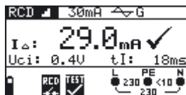
Fig. 5.20: Example of trip-out current measurement result
