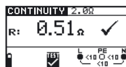
Fig. 5.12: Example of Continuity measurement result
