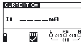
Fig. 5.47: TRUE RMS current measurement menu
