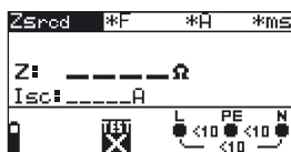
Fig. 5.31: Loop impedance measurement menu
