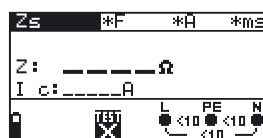
Fig. 5.28: Loop impedance measurement menu
