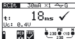
Fig. 5.18: Example of trip-out time measurement results
