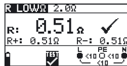
Fig. 5.8: Example of Low \Omega resistance measurement results
