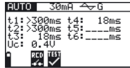
Fig. 5.25: Step 4 RCD autotest results
