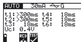
Fig. 5.27: Step 6 RCD autotest results
