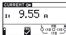
Fig. 5.49: Example of TRUE RMS current measurement result
