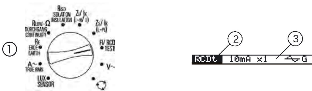
Fig. 4.2: Function selector switch and respective parameter line, example: BENNING IT 120 B
