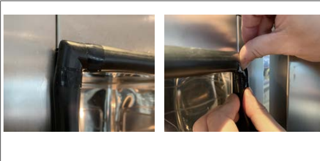
Image: Insert seal at the top corners first
