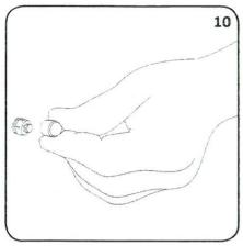
Tighten the nut with a spanner and allen key. Place ITEM 13 onto of fixings, securing the cup the nut.
