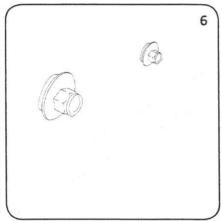
Place ITEM 5 on to ITEM 6. From the inside of the bin, push through one of the two fixing holes at the base of the bin body. Place ITEM 7, 8 and 9 onto the Screw from the outside of the body.
