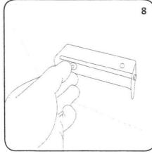
Align ITEM 11 over the top fixing holes on the outside of the Nexus Body place the washer M6 x 100. Place the screw M6 x20mm through one of the fixing holes.
