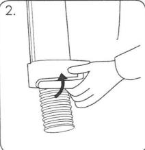
To remove the cups, move the quick release 45 degrees to the right.
