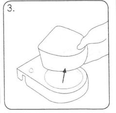
To empty or clean, remove the drip tray from the drip tray bracket.
