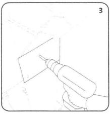
Place ITEM 1 in place on the right Lay the bin body on its side, drill hand side of the bin body. Align the template with the holes in the body and poke through with a pencil. Use 2 x ITEM 2 & ITEM 3 to temporarily fix the template to the bin.
