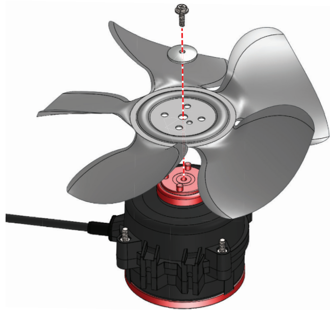
Fig. 14. Be sure the washer slopes down and away from the center of the fan motor.
